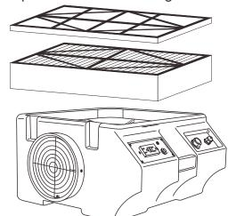
The filter is the same size as the pleated fabric filter. Install it in place of the pleated fabric filter.
